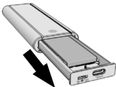
2. Insert the M.2 SSD at an angle of about 30°, carefully press the M.2 SSD down and secure it with the rubber fixation. Install a thermal pad on the M.2 SSD and place the heat sink on it.
