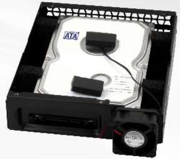
Temperature controlled fan and vibration absorption foam
