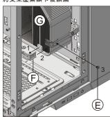
The bracket can also be installed in reverse when using a thinner graphics card.
