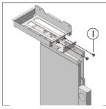
Install the tray back. 將托盤安裝回去
