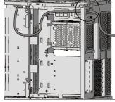
GPU output cable routing.
