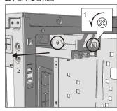
Install GPU on the tray and plug the output cable
