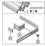
Height adjustable according to the GPU length and the power connection position.
