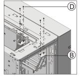
Installation for GPU mount at the first slot.
