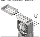
Install water cooling GPU on the tray and plug the output cable.
