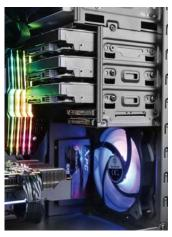
Precisely designed space capable of accommodating various storage devices (5.25" / 3.5" / 2.5") with dual USB 3.0 ports
