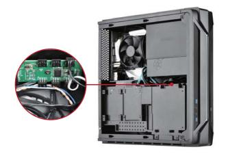
Install graphics card support bracket into the chassis and connect the power cord to the graphics card if needed
