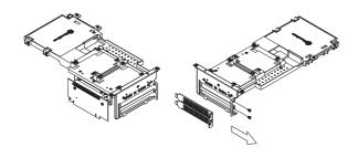
Depending on the design of your graphics cards, install and adjust the graphics card holder to a proper position to support your card. Adhere included rubber padding according to the height of graphics card's backside, one (for 3mm thick backplate) or two (for no backside components)
