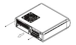
Unscrew the screws from the graphics card support bracket then remove it
