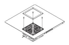
The graphics card holder needs to be removed before dismounting the fans on the bottom vents We recommend removing the filters before dismounting the fans
