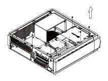
Unscrew the screws from PSU bracket then remove it
