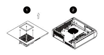
Insert the I/O shield included with your motherboard then install the motherboard into the chassis
