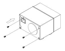
Place the PSU bracket on top of the chassis then connect the power cord to the PSU
