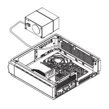
Insert the PSU bracket into its original position and secure with screws
