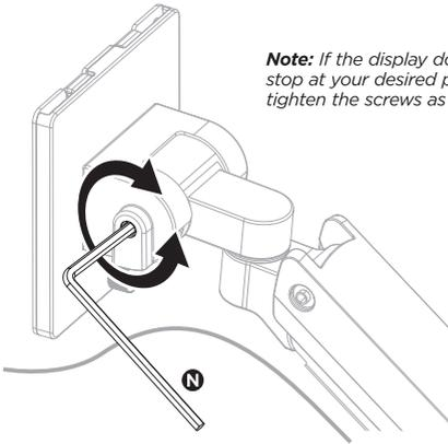
**Note:** If the display does not stop at your desired position, tighten the screws as shown.
