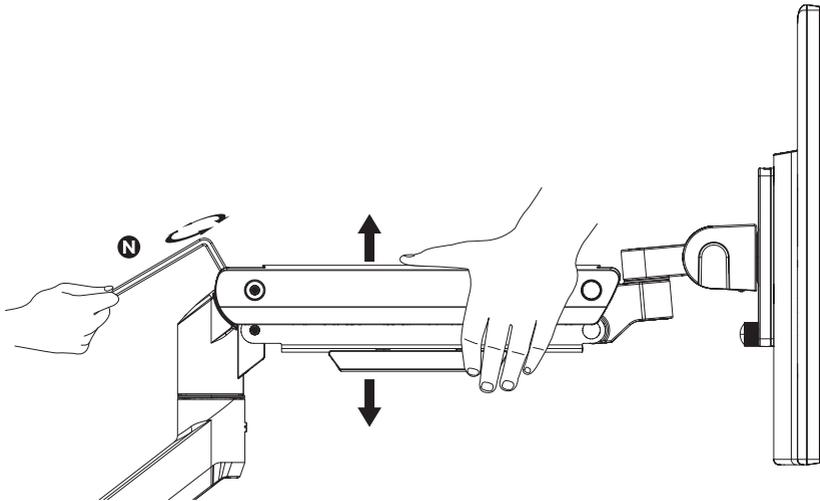
To properly balance the arm with monitor mounted, adjust the spring tension using the supplied Allen Key as follows:
