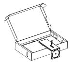
Use a screwdriver to remove the base screws.
