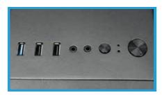
TOP PANEL I/O Ample USB ports, including HD audio and mic. with easy access to reset and rounded power button.
