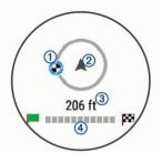
The destination indicator ① shows the direction of your destination relative to the direction you are moving ②. When the destination indicator appears at the top of the circle, you are heading toward your destination. The remaining distance to your destination ③ appears below the circle. The progress bar ④ shows your progress toward your destination.
