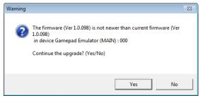
If you didn't enable *Check Firmware Version*, the Utility installs the upgrade files without checking whether they are a higher level, or not.
