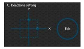
The Deadzone is a small area around the *Right Stick* control that doesn't respond to movement. Movement only occurs when the *Right Stick* moves outside the Deadzone. Each game sets its own Deadzone size. The Deadzone affects mouse movements. With no Deadzone there is no delay with the mouse and movements are very straight and accurate.
