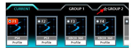
5. Use the **Radio Button** to set the default start-up profile (turns red). This is the default profile that will be selected for use when the Phantom-S is connected to the game console
