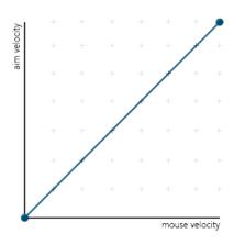
**Mouse Velocity** increases from left to right. **Aim Velocity** increases from bottom to top. As you adjust the curve up and down, the relationship of physical mouse speed to on-screen speed changes. The two sections represent different movements:
