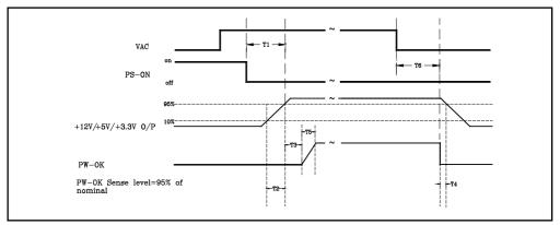
Figure 2. PS-OK Timing Sequence
