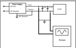
Figure 1. Ripple voltage test circuit
